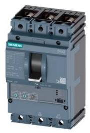
CIRCUIT BREAKER 3VA2 IEC FRAME 250 BREAKING CAPACITY CLASS C ICU=110KA @ 415 V 3POLE, LINE PROTECTION ETU320, LI, IN=250A OVERLOAD PROTECTION IR=100A ...250A SHORT CIRCUIT PROTECTION II=10 X IN BUSBAR CONNECTION
