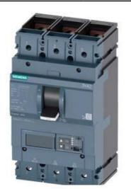
CIRCUIT BREAKER 3VA2 IEC FRAME 400 BREAKING CAPACITY CLASS C ICU=110KA @ 415 V 3-POLE, LINE PROTECTION ETU860, LSIG, IN=400A OVERLOAD PROTECTION IR=160A ...400A SHORT CIRCUIT PROTECTION ISD=0,6..10X IN, II=1,5..10X IN NEUTRAL PROTECTION OPTIONAL WITH EXT. CT;UPTO 160% GROUND-FAULT, SWITCHABLE IG=0,2... 1 X IN, TG=0,05-0,8MS BUSBAR CONNECTION
