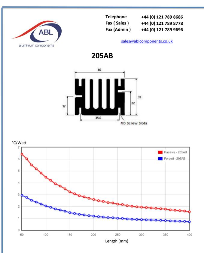
Thermal Resistance is calculated based on a distributed heat load and vertically mounted fins anodised heatsink with a 60°C temperature.
