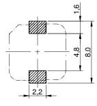
no sensitive traces underneath the component
