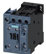
power contactor, AC-3, 32 A, 15 kW / 400 V, 4-pole, 24 V DC, auxiliary contacts: 1 NO + 1 NC, screw terminal, size: S0
