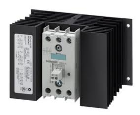
SOLID-STATE CONTACT.3PHASE 3RF2 AC51 40A 40 DEG. C 48-600V / 110V AC 3-PHASE CONTROLLED SCREW TERMINAL BLOCKING VOLTAGE 1200V
