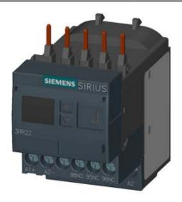
MONITORING RELAY ATTACHABLE TO CONTACTOR 3RT2. SIZE S00 STANDARD, DIGITAL ADJUSTABLE APPARENT/ACTIVE CURRENT MONIT. 1.6 - 16A, 20-400 HZ, 3-PHASE SUPPLY 24-240 V AC/DC 1 CO CONTACT, 1 SEMICOND. FOR ALARM AND WARNING MONITORING FOR CURRENT OVERSHOOT/UNDERSHOOT PHASE FAILURE, WIRE BREAK PHASE SEQUENCE FAULT CURRENT BLOCKING CURRENT WARNING AND ALARM THRESHOLDS WITH OR W/O ERROR LOG ONDELAY 0-99 S SPURIOUS PEAK SUPPR. 0-30 S BREAK AFTER FAULT 0-300 MIN SCREW CONNECTION
