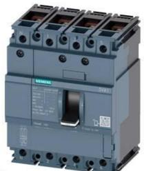
CIRCUIT BREAKER 3VA1 IEC FRAME 160 BREAKING CAPACITY CLASS N ICU=25KA @ 415 V 4-POLE, LINE PROTECTION TM210, FTFM, IN=32A OVERLOAD PROTECTION IR=32A FIXED SHORT CIRCUIT PROTECTION II=10 X IN NEUTRAL UNPROTECTED BUSBAR CONNECTION
