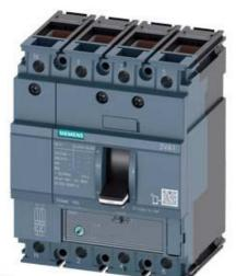
CIRCUIT BREAKER 3VA1 IEC FRAME 160 BREAKING CAPACITY CLASS S ICU=36KA @ 415 V 4-POLE, LINE PROTECTION TM220, ATFM, IN=32A OVERLOAD PROTECTION IR=22,4A ...32A SHORT CIRCUIT PROTECTION II=10 X IN NEUTRAL PROTECTION 100% CABLE CONNECTION
