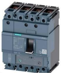
CIRCUIT BREAKER 3VA1 IEC FRAME 160 BREAKING CAPACITY CLASS M ICU=55KA @ 415 V 4-POLE, LINE PROTECTION TM240, ATAM, IN=16A OVERLOAD PROTECTION IR=11,2A ...16A SHORT CIRCUIT PROTECTION II=5...10 X IN NEUTRAL UNPROTECTED BUSBAR CONNECTION
