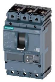
CIRCUIT BREAKER 3VA2 IEC FRAME 160 BREAKING CAPACITY CLASS M ICU=55KA @ 415 V 3POLE, LINE PROTECTION ETU850, LSI, IN=40A OVERLOAD PROTECTION IR=16A ...40A SHORT CIRCUIT PROTECTION ISD=0,6..10X IN, II=1,5..12X IN NEUTRAL PROTECTION OPTIONAL WITH EXT. CT,UPTO 160% BUSBAR CONNECTION
