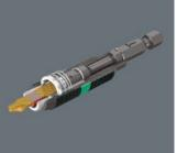
The effectiveness of the BiTorsion system comes from a combination of two shock-absorbing spring elements. Both bits as well as holders have a cushioning torsion zone that diverts the kinetic energy away from the drive tip during peak loads.
