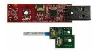
The Si705x temperature sensor evaluation kits and accompanying graphical user interface software allow quick and easy access to the features and functions of the <u>Si705x temperature</u> <u>sensor family</u> while enabling the evaluation of the sensor's performance. Four different kits are available, depending on the accuracy desired.
