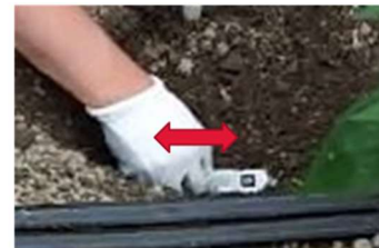
③ Put sensor with sticking to soil, then move right/left for more close sticking
