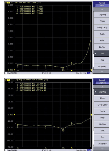
VSWR and Return Loss Model: ANT-868-10dbi-Yagi 6 Elements
