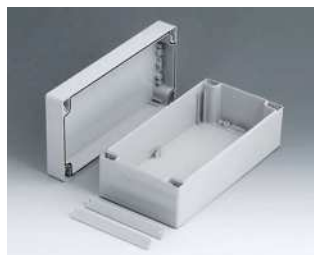
C2112242 ROBUST-BOX 120 BREIT, Ausf. II PC (UL 94 HB) lichtgrau RAL 7035 240x120x90mm IP 66
