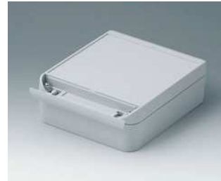
C6015181 SMART-BOX 150 BREIT ASA+PC-FR (UL 94 V-0) lichtgrau RAL 7035 180x150x60mm IP 66
