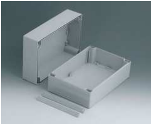
C2416241 ROBUST-BOX 160 BREIT, Ausf. I ABS (UL 94 HB) lichtgrau RAL 7035 240x160x120mm IP 66
