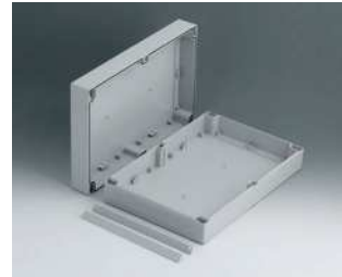
C2120301 ROBUST-BOX 200 BREIT, Ausf. I ABS (UL 94 HB) lichtgrau RAL 7035 300x200x80mm IP 66
