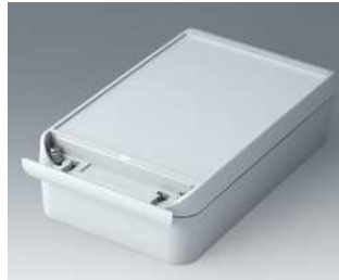
C6013221 SMART-BOX 130 BREIT ASA+PC-FR (UL 94 V-0) lichtgrau RAL 7035 220x130x60mm IP 66
