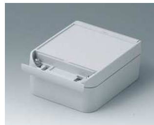
C6011141 SMART-BOX 110 BREIT ASA+PC-FR (UL 94 V-0) lichtgrau RAL 7035 140x110x60mm IP 66
