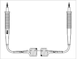
The meter start-up tester – double insulated coil cable with 2 test probes – generates a resistive load of 705  $\Omega$  which loads the energy meter with approximately 75 W at a line voltage of 230 V. Overload capacity: 440 V. The test instrument is supplied with a convenient carrying case.
