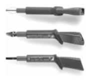
Three self-retaining, contactprotected test probes for the connection of measurement cables with 4 mm banana plugs or with contact-protected plugs to 3.5 to 12 mm outlets, e.g. CEE outlets, Perilex outlets etc. For example, the test probes fit into the square PE sockets at Perilex outlets. Maximum allowable operating voltage: 600 V per IEC 61010.
