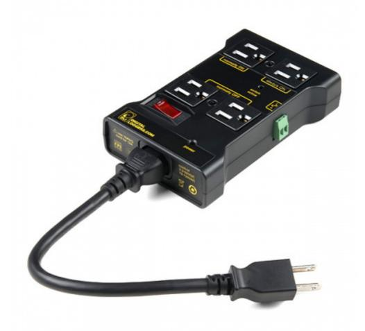
The IoT Power Relay is designed to allow you to safely control an outlet device that operates at 3--48VDC or 12--120VAC. Each IoT Power Relay features a single input (from the included C13 power cable) to four outputs: one normally on, one always on, and two normally off. The durable SPDT control relay is rated at 30/40A, for 400,000 operations.
