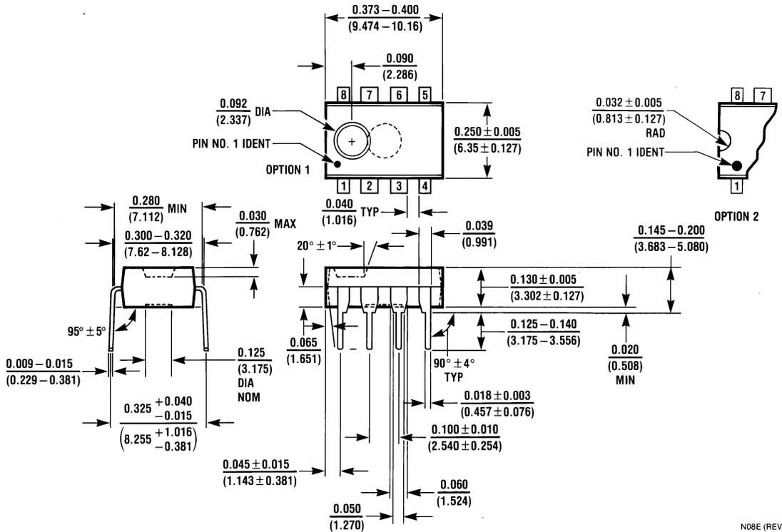
**8-Lead (0.300" Wide) Molded Dual-In-Line Package,
