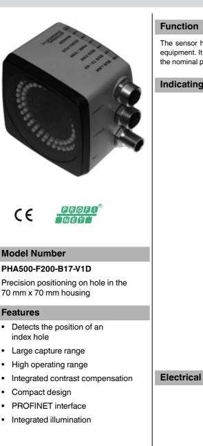
The sensor has been developed for the precision positioning of high-bay racking operating equipment. It detects circular holes in the racking structure and their positional deviation from the nominal position. The sensor operates in two dimensions.
