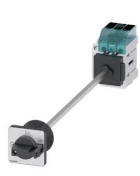
Switch disconnector 3LD3, main switch 3-polig, lu 32A operational switch at AC-23 A at 400 V 11,5 kW floor mounting Base mounting with door coupling center-hole 22,5 mm knob-operated mechanism black 48 x 48 mm with auxiliary 1NO+1NC
