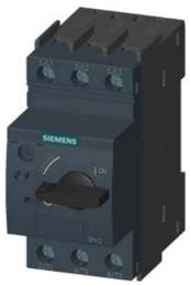
SPECIAL TYPE CIRCUIT BREAKER SIZE S00, FOR MOTOR PROTECTION, CLASS 10, A-RELEASE 7...10A, SHORT-CIRCUIT RELEASE 130A, SCREW TERMINAL, STANDARD SWITCHING CAPACITY AMBIENT TEMPERATURE -50 DEGREES C 500 SWITCHING CYCLES
