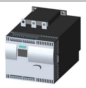
SIRIUS SOFT STARTER, VALUES WITH 690 V, 40 DEG., STANDARD: 113A, 110KW, INSIDE-DELTA CIRCUIT 3: ONLY UP TO 600V, 400-690 V AC, 230 V AC, SCREW TERMINALS
