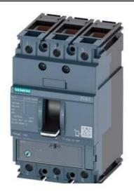
CIRCUIT BREAKER 3VA1 IEC FRAME 160 BREAKING CAPACITY CLASS H ICU=70KA @ 415 V 3-POLE, LINE PROTECTION TM220, ATFM, IN=40A OVERLOAD PROTECTION IR=28A ...40A SHORT CIRCUIT PROTECTION II=10 X IN CABLE CONNECTION
