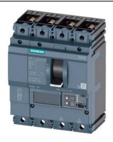
CIRCUIT BREAKER 3VA2 IEC FRAME 160 BREAKING CAPACITY CLASS C ICU=110KA @ 415 V 4POLE, LINE PROTECTION ETU560, LSIG, IN=160A OVERLOAD PROTECTION IR=64A ...160A SHORT CIRCUIT PROTECTION ISD=0,6..10X IN, II=1,5..10X IN NEUTRAL PROTECTION ADJUSTABLE (OFF, UPTO 100%) GROUNDFAULT, SWITCHABLE IG=0,2... 1 X IN, TG=0,050,8MS BUSBAR CONNECTION
