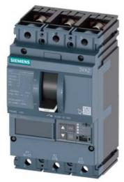
CIRCUIT BREAKER 3VA2 IEC FRAME 160 BREAKING CAPACITY CLASS C ICU=110KA @ 415 V 3POLE, LINE PROTECTION ETU850, LSI, IN=63A OVERLOAD PROTECTION IR=25A ...63A SHORT CIRCUIT PROTECTION ISD=0,6..10X IN, II=1,5..12X IN NEUTRAL PROTECTION OPTIONAL WITH EXT. CT,UPTO 160% BUSBAR CONNECTION
