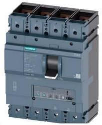
CIRCUIT BREAKER 3VA2 IEC FRAME 400 BREAKING CAPACITY CLASS H ICU=85KA @ 415 V 4-POLE, LINE PROTECTION ETU330, LIG, IN=250A OVERLOAD PROTECTION IR=100A ...250A SHORT CIRCUIT PROTECTION II=1,5...12 X IN NEUTRAL PROTECTION ADJUSTABLE(OFF,50%,100%) GROUND-FAULT-PROTECTION IG=0,2... 1 X IN, TG=0,1/0,3MS BUSBAR CONNECTION
