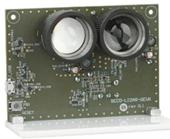
The kit is FDA certified and includes a multifunctional GUI enabling a complete evaluation of the range-finding performance as well as the adjustment of system variables such as the buffer number of pulses or the bias voltage for the SiPM-RB photomultiplier.
