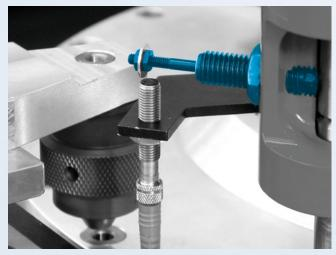
The tools are also available with an actuating bolt that is protected against rotating.
