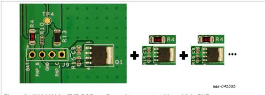
Figure 8. UJA1169Ax-EVB PCB configured to operate with multiple PNPs.
