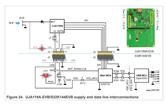
A 12 V power supply must be connected to header J2 or to jack J6 on the UJA1169A-EVB (see also <u>Figure 19</u>). It supplies the BAT pin of the SBC via a polarity protection diode.
