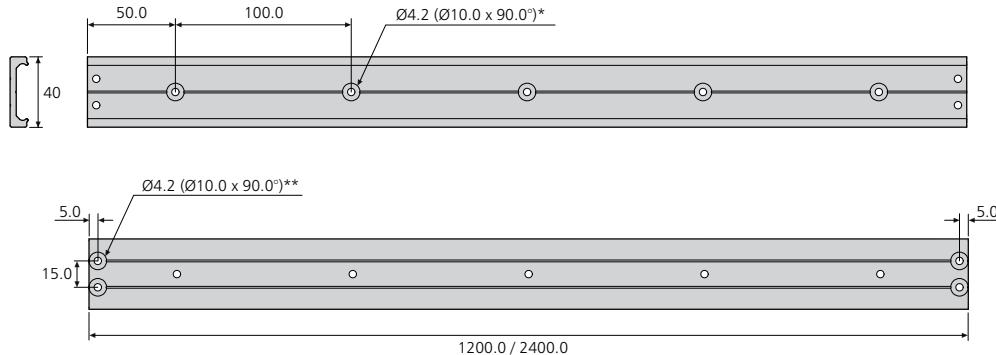
\* Fixing: drill 4.2mm holes on centre line, fully countersunk.
