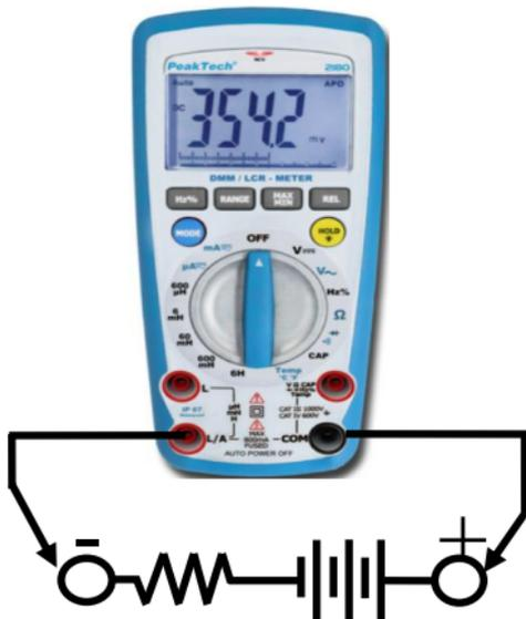
1. Set the rotary selector to the desired  $\mu\text{A}$  or  $\text{mA}$  - range. If you do not know the current level, set it to the highest position and reduce the setting as needed to get a reading.
