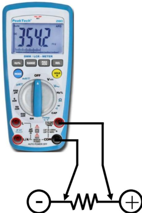
The resistance measuring circuit compares the voltage gained through a known resistance (internal) with the voltage developed across the unknown resistance. So, when you check in-circuit resistance, be sure the circuit under test has all power removed (all capacitors are fully discharged).
