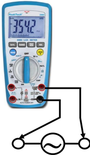
**Warning!** When you connect the test probes to an AC outlet/ mains voltage , do not turn the rotary selector switch to another range. It could damage the meter's internal components or injure you.
