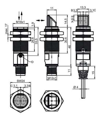
A Vertical position of the optical axis
