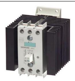
SEMI-CONDUCTOR CONTAC.3-PH.3RF2 AC51 20A 40 DEG. C 48-600V / 4-30V DC 3-PHASE CONTROLLED SCREW TERMINAL BLOCKING VOLTAGE 1200V
