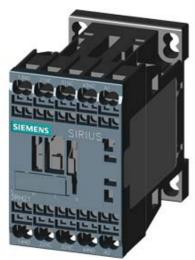
CONTACTOR RELAY, 2NO+2NC, AC 230V, 50/60 HZ, SZ S00, SPRING-LOADED TERMINAL
