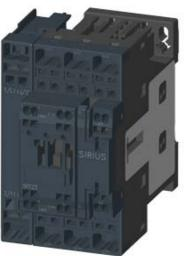
4NO CONTACTOR, AC1: 40A AC 24V 50/60HZ 4-POLE, 4NO, SZ: S0, SPRING-LOADED TERMINAL 1NO+1NC INTEGR.
