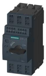
CIRCUIT-BREAKER SZ S00, FOR MOTOR PROTECTION, CLASS 10, A-REL. 0.18...0.25A, N-RELEASE3.3A SPRING-L. CONNECTION STANDARD SW. CAPACITY W. TRANSVERSE AUX. SWITCH 1NO+1NC
