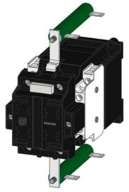
CONTACTOR SIZE 2, 2-POLE, FOR RAILWAY APPLICATIONS DC-3 AND 5, 7.5A AT 750V AUX. CONTACTS 21 (2NO+1NC) OPERATING RANGE 0.7...1.25 X US WITH VARISTOR AND SERIES RESISTOR DC SOLENOID SYSTEM 33V DC
