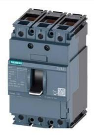
CIRCUIT BREAKER 3VA1 IEC FRAME 100 BREAKING CAPACITY CLASS B ICU=16KA @ 415 V 3-POLE, LINE PROTECTION TM210, FTFM, IN=80A OVERLOAD PROTECTION IR=80A FIXED SHORT CIRCUIT PROTECTION II=10 X IN CABLE CONNECTION
