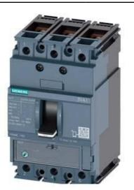
CIRCUIT BREAKER 3VA1 IEC FRAME 160 BREAKING CAPACITY CLASS M ICU=55KA @ 415 V 3-POLE, LINE PROTECTION TM220, ATFM, IN=40A OVERLOAD PROTECTION IR=28A ...40A SHORT CIRCUIT PROTECTION II=10 X IN BUSBAR CONNECTION
