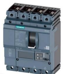
CIRCUIT BREAKER 3VA2 IEC FRAME 100 BREAKING CAPACITY CLASS L ICU=150KA @ 415 V 4POLE, LINE PROTECTION ETU550, LSI, IN=100A OVERLOAD PROTECTION IR=40A ...100A SHORT CIRCUIT PROTECTION ISD=0,6..10X IN, II=1,5..12X IN NEUTRAL PROTECTION ADJUSTABLE (OFF, UPTO 100%) BUSBAR CONNECTION
