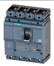
CIRCUIT BREAKER 3VA2 IEC FRAME 160 BREAKING CAPACITY CLASS L ICU=150KA @ 415 V 4POLE, LINE PROTECTION ETU320, LI, IN=100A OVERLOAD PROTECTION IR=40A ...100A SHORT CIRCUIT PROTECTION II=12 X IN NEUTRAL PROTECTION ADJUSTABLE(OFF,50%,100%) BUSBAR CONNECTION
