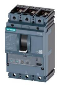
CIRCUIT BREAKER 3VA2 IEC FRAME 160 BREAKING CAPACITY CLASS H ICU=85KA @ 415 V 3POLE, LINE PROTECTION ETU350, LSI, IN=40A OVERLOAD PROTECTION IR=16A ...40A SHORT CIRCUIT PROTECTION ISD=1,5... 10 X IR, II=12 X IN BUSBAR CONNECTION
