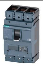
CIRCUIT BREAKER 3VA2 IEC FRAME 630 BREAKING CAPACITY CLASS H ICU=85KA @ 415 V 3-POLE, LINE PROTECTION ETU560, LSIG, IN=400A OVERLOAD PROTECTION IR=160A ...400A SHORT CIRCUIT PROTECTION ISD=0,6..10X IN, II=1,5..15X IN NEUTRAL PROTECTION OPTIONAL WITH EXT. CT;UPTO 160% GROUND-FAULT, SWITCHABLE IG=0,2... 1 X IN, TG=0,05-0,8MS BUSBAR CONNECTION
