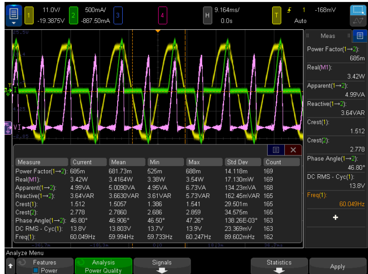
Figure 1. Input AC power quality measurements.
