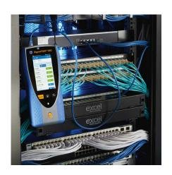
The SignalTEK 10G will log all network events over a 72-hour period to help diagnose connectivity issues faster, reducing hours onsite and reducing trips to site.
