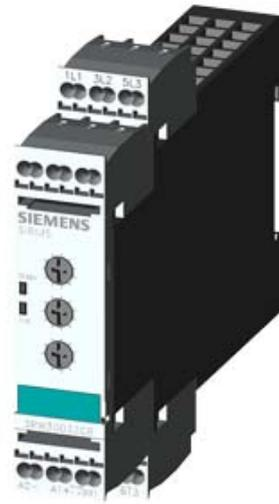
SIRIUS SANFTSTARTER, 22,5 MM, 3A, 1,1KW/400V, 40GRAD, AC 200-400V, AC/DC 24-230V, FEDERZUGKLEMMEN
