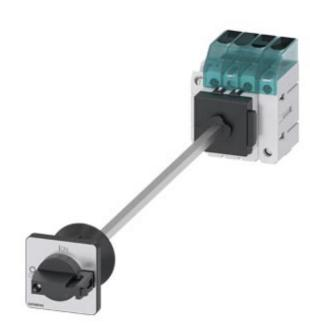
Switch disconnector 3LD3, main switch 3-polig + N, lu 25A operational switch at AC-23 A at 400 V 9,0 kW floor mounting Base mounting with door coupling center-hole 22,5 mm knob-operated mechanism black 48 x 48 mm with auxiliary 1NO+1NC
