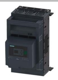
FUSE-SWITCH-DISCONNECTOR 3-POLE, NH00, 160A 60MM BUSBAR SYSTEM COVER LEVEL 32/70 MM FLAT CONNECTOR FUSE MONITORING ELECTRONIC, EFM 20
