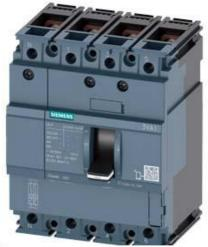
CIRCUIT BREAKER 3VA1 IEC FRAME 160 BREAKING CAPACITY CLASS N ICU=25KA @ 415 V 4-POLE, LINE PROTECTION TM210, FTFM, IN=20A OVERLOAD PROTECTION IR=20A FIXED SHORT CIRCUIT PROTECTION II=10 X IN NEUTRAL PROTECTION 100% BUSBAR CONNECTION
